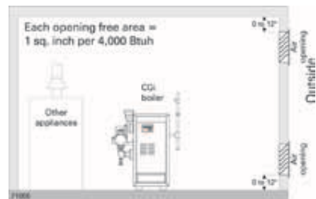
Figure 4 Air from outdoors — vertical ducts
