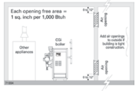
Figure 2 Air openings to interior spaces
